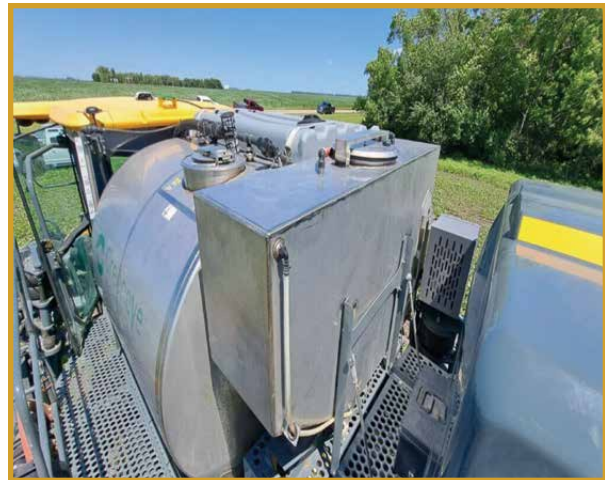
Figure 2: A smaller spot spray tank was added to the Hagie. If necessary, spray mix can be pumped from the larger tank to this smaller tank.
