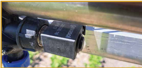
Figure 5: Solenoids activate the spray when a weed is detected in that nozzle's lane.
