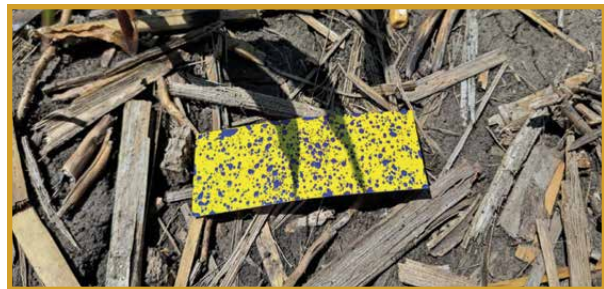
Figure 8: The spray deposit shows adequate coverage and a good droplet size distribution for good placement accuracy.
