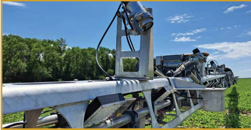
Figure 9: The camera and lights look ahead to provide the necessary time for the on-board computer to make the required calculations that determines the plant's identity. Note the aspirated lens cleaner.
