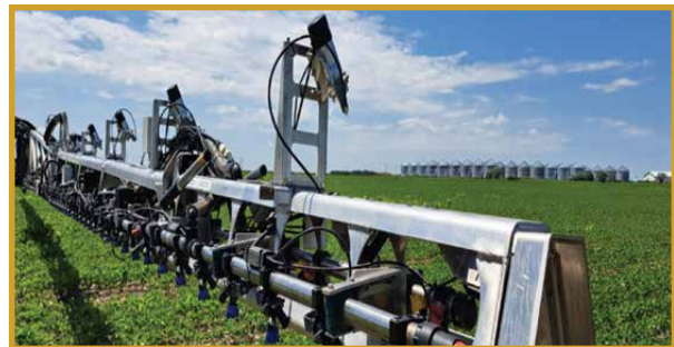
Figure 3: The second (spot spray) boom is mounted behind the factory wet boom.
