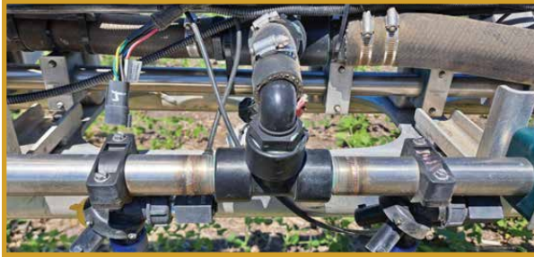
Figure 4: The spot spray nozzles are mounted at 10" (25 cm) spacing.
