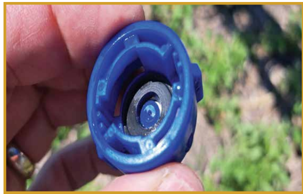
Figure 7 (bottom): The blue DG pre-orifice meters the flow at 0.3 US gpm at 40 psi.
