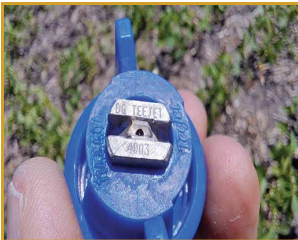
Figure 6: These Drift Guard nozzles are custom-made for Greeneye by TeeJet. Figure 6 (top): These Drift Guard nozzles are custom-made for Greeneye by TeeJet.
