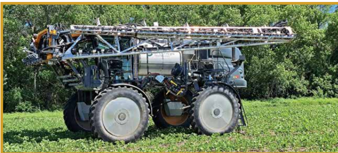
Figure 1: The Greeneye system was mounted on a Hagie STS 12 sprayer.
